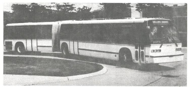
Adding to our special APTA/IPTE report (*TC 10-30 October 1981*) is this view of GMC's new articulated RTS. The 56-foot coach seats up to 65 (73 in the 61-foot version), and is available with either two or three doors, but is not expected to be in production until 1984. The unit is an articulated version of the Advanced Design Series "04" RTS coach.
