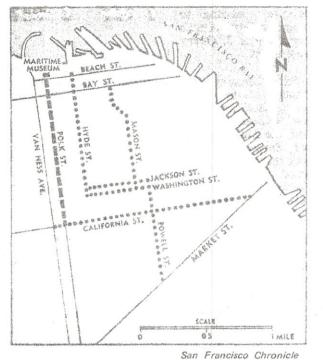
Existing cable lines are shown by dots. Proposed California Street cable extension is shown by heavy dashed line. Route extension would cut overloading on Powell Street lines and lessen auto traffic in Fisherman's Wharf area (near Maritime Museum on map).
