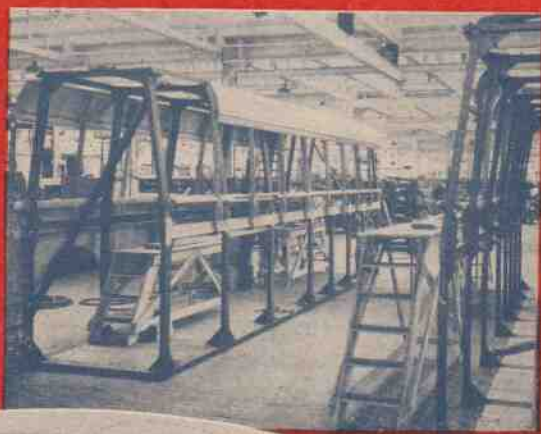
Supporting framework of the bus is of curved metal design and is incredibly strong though light in weight.
