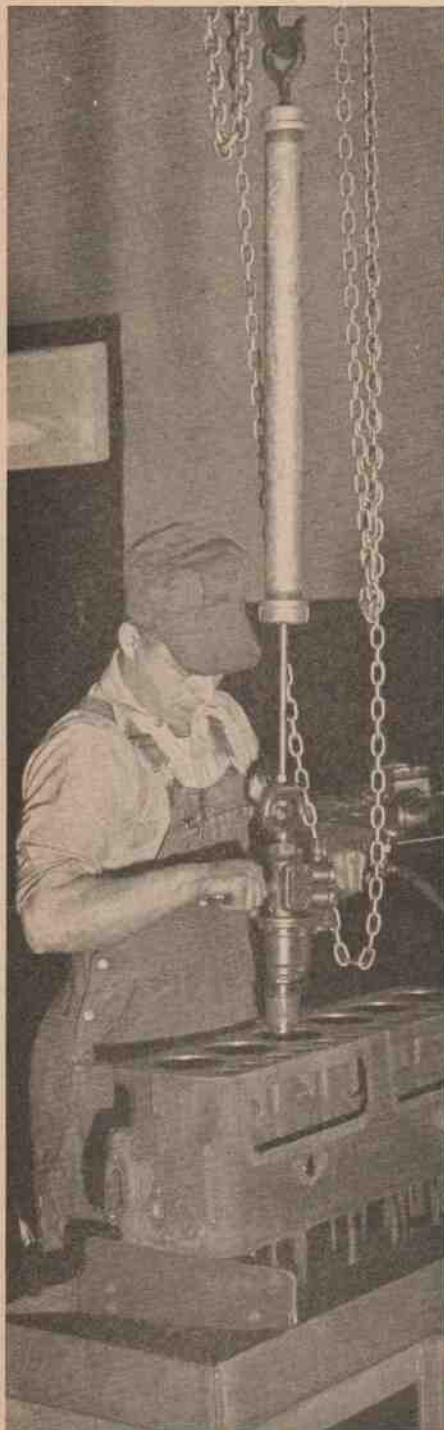
This new method of suspending a cylinder hone was devised—and is demonstrated—by Walter Olenick. As a result of this suggestion the job is done much easier, safer, and efficiently.
